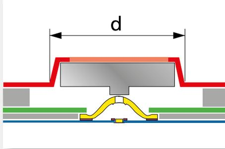
The back-lit Profiline keypad has additional advantages such as its long operating life, low power consumption and haptic. This technology makes it possible to illuminate the keys separately and the light passes through a hole in the special snap dome into the integrated acrylic inlay, where it is scattered accordingly.
