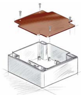
Standard mounting panel fixing, in part also in the lid.
