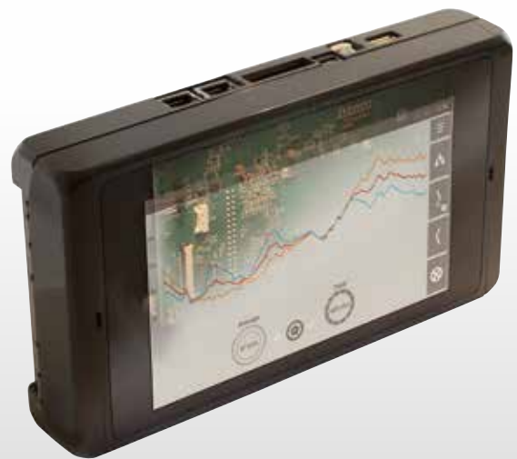
Bocube With back-printed glass plate, bonded touch screen / display unit + SBC.
