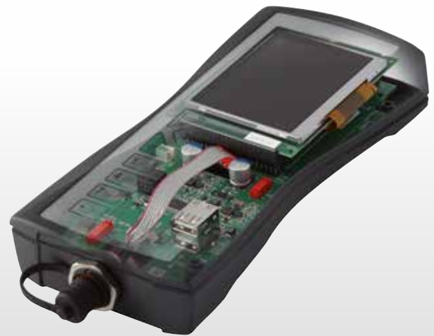
BOS-Streamline Display combined with customised membrane keypad.
