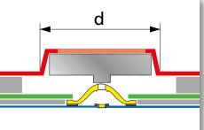
The back-lit Profiline keypad has additional advantages such as its long operating life, low power consumption and haptic. This technology makes it possible to illuminate the keys separately and the light passes through a hole in the special snap dome into the integrated acrylic inlay, where it is scattered accordingly.
